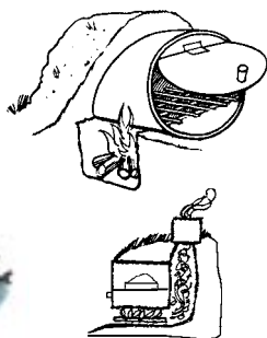
Traditional clay oven - barrel bridges fire pit, chimney constructed of tin cans
