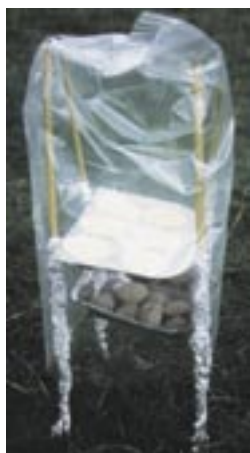
Turkey bag stove works on the same principle as cardboard box stove and uses charcoal
