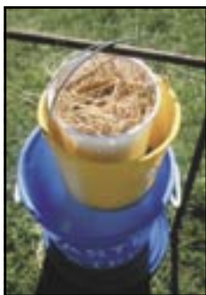
Waste water filter system
