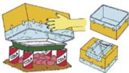
Cardboard box stove. Line a box with tin foil. Leave a small gap under edge of box to allow air in. The average temperature of an individual coal is 20 degrees. Place inside the box the number of coals required to make up temperature as stated in recipe.
